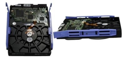
The HDD rail should look like this when place correctly with Hard Drive.
